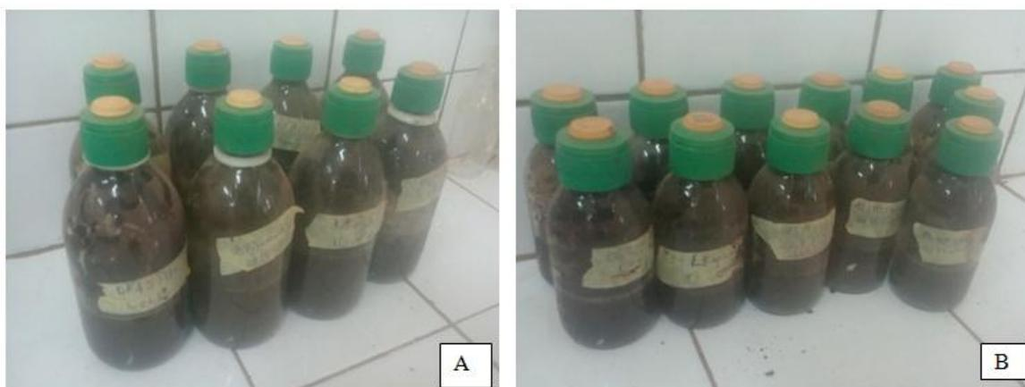
**Figure 1:** Digesters for biomethanization used in the study. A: 250 ml septum vials; B: septum vials of 120 ml.
