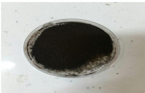
**Figure 2:** The synthesis of Copper oxide nanoparticles by using green method
